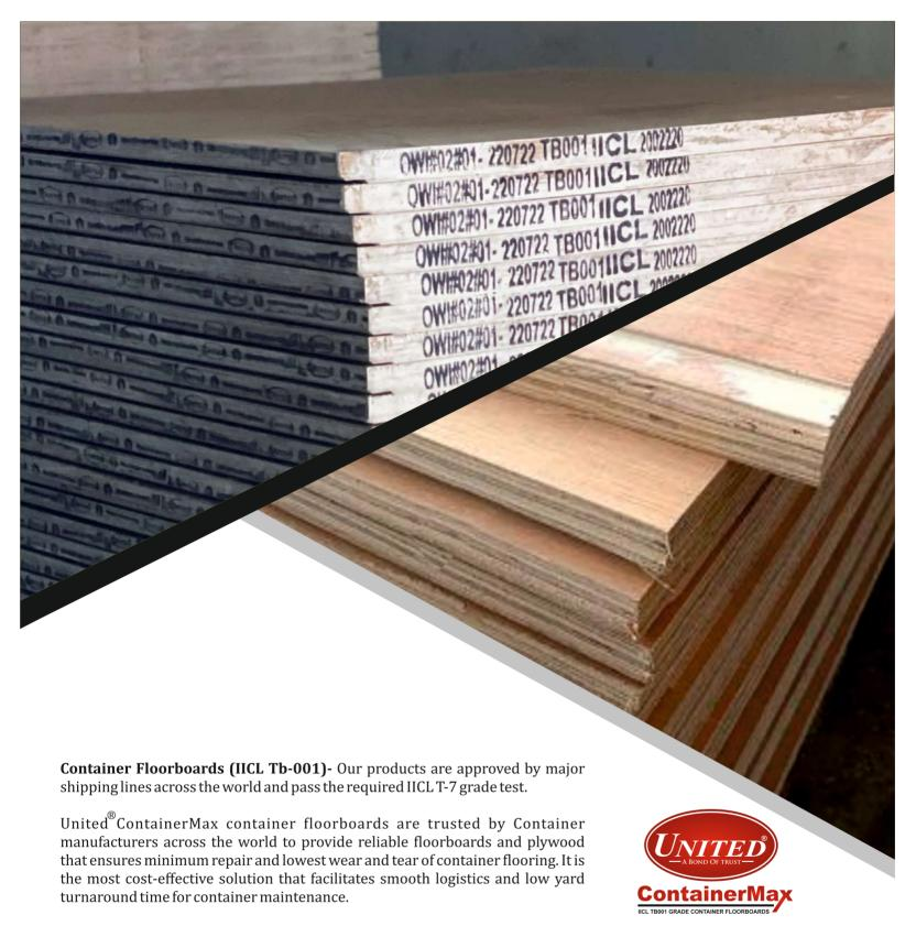
Available in 28mm, 19+2 Layer construction, groove as per design & black phenolic waterproof film to protect the container floor from the bottom.
